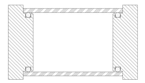
OD O-rings also work well but beware that the tolerance on the cylinder OD is large (+/-.010" typically). Also, the ID/OD concentricity of the cylinder can be several thousandths, which can be important if precise locating is needed. That said, OD O-rings work great for prototypes because the OD of the cylinder can be measured and then the gland for the O-ring could be made to fit. Again, use P-80<sup>TM</sup>.
