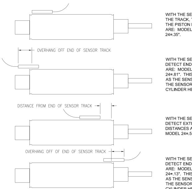
WITH THE SENSOR FLUSH TO THE REAR END OF THE TRACK, THE SENSOR WILL SWITCH BEFORE THE PISTON BOTTOMS OUT. TYPICAL DISTANCES ARE: MODEL 9=.12", MODEL 16=.23", MODEL 24= 35"
